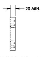
NOTE: THICKER THAN 20mm PLATE IS RECOMMENDED TO INCLUDE A PILOT BORE FOR THE CATHODE.
