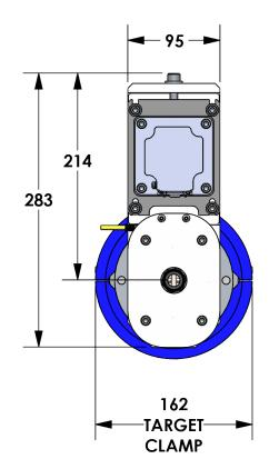
ABSOLUTE MINIMUM DRIVESHAFT LENGTH = WALL THICKNESS +20mm
